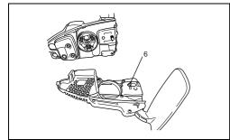
Turn the chain adjusting screw (5) to the left (counterclockwise) until the pin (6) is at the right stop.
